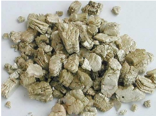
Processed vermiculite often seen as insulation.
