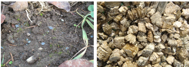
(Left) Raw vermiculite in soils. (Right) When heated, vermiculite exfoliates (or pops), forming a lightweight material ideal for packing, insulation, and as a soil additive.
