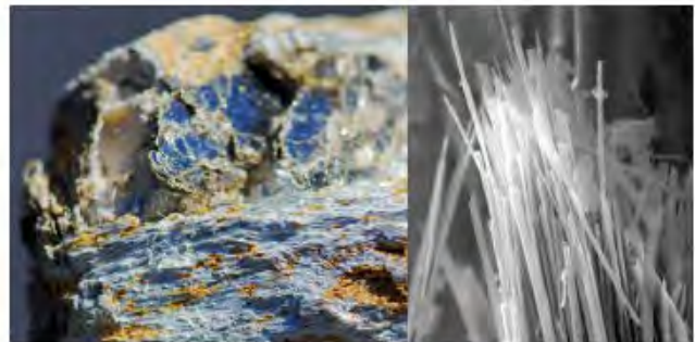
Libby Amphibole asbestos with vermiculite ore in raw form (L) and asbestos fibers (magnified) (R)
