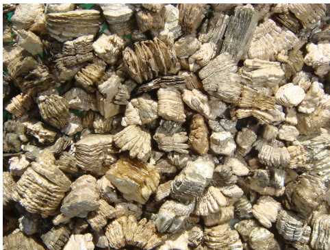
Processed vermiculite often seen as insulation
